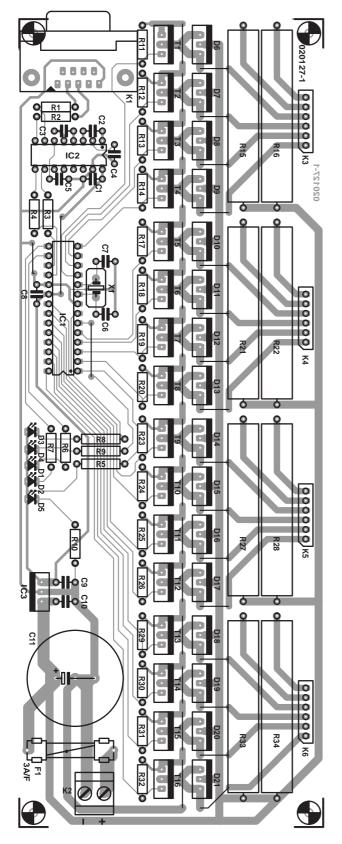
Figure 3. PCB design for the stepper motor driver board.
