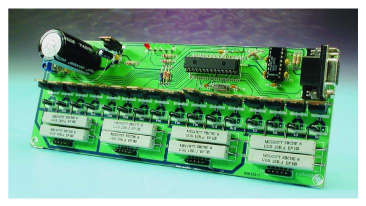
Figure 5. Our finished prototype of the stepper motor driver.
