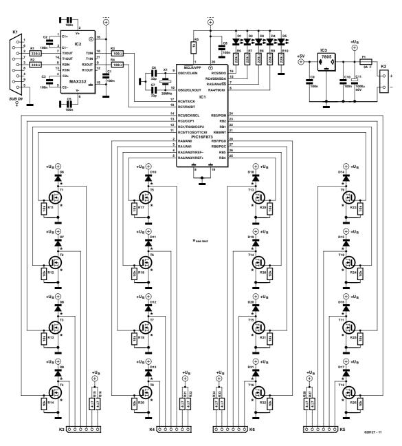
Figure 2. Circuit diagram of the driver board.
