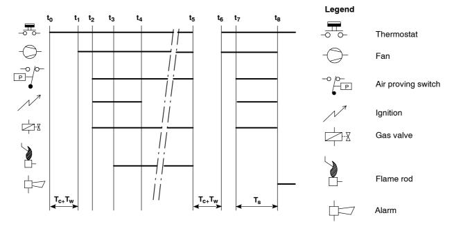
Fig. 11. Functional diagram S4565CM, DM, RM,TM
