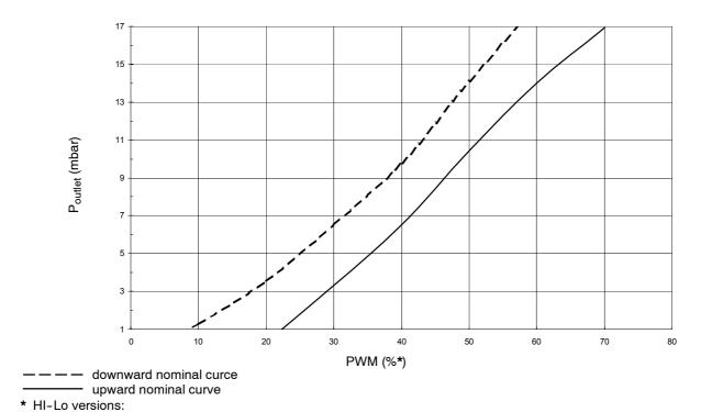
Fig. 2. Nominal graph modulating performance at 20 mbar inlet pressure,  $\varnothing$  4.3 mm outlet restriction
