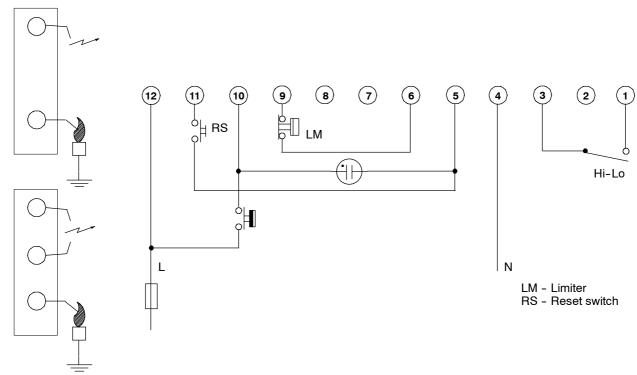
Fig. 8. Connection diagram S4565BM, QM with Hi-Lo 1)
