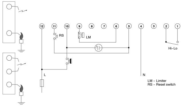
Fig. 6. Connection diagram S4565AM, PM with Hi-Lo 1)
