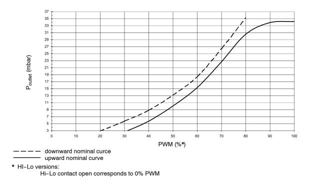
Fig. 3. Nominal graph modulating performance at 37 mbar inlet pressure,  $\varnothing$  2.8 mm outlet restriction
