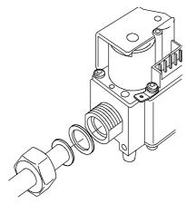
Fig. 12. External thread G<sup>1</sup>/<sub>2</sub>" connection with nut and flat sealing ring
