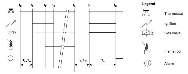
Fig. 10. Functional diagram S4565AM, BM, PM, QM
