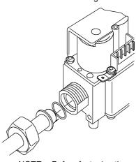
NOTE: Before fastening the nut be sure that the "O"-ring is proper placed on the pipe.
