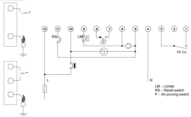
Fig. 9. Connection diagram S4565DM, TM with Hi-Lo 1)
