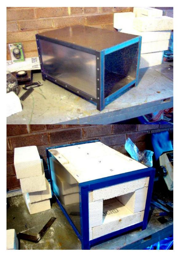
Fit your firebricks in the case, working from the centre outwards and then cutting the bricks to fit. You should end up having to cut bricks about 35mm wide on either side. The brick are VERY easy to cut with an ordinary handsaw used for wood. I have also used a hacksaw blade for trimming and carving the grooves.
