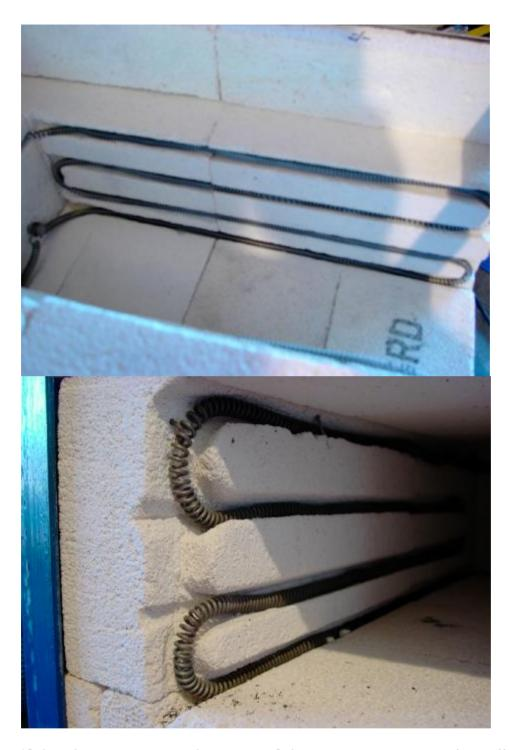
If the elements want to jump out of the grooves you can push small pins bent in the shape of hair pins or horse shoes! Around the element and into the firebrick. This is why you need the soft bricks!!!!
