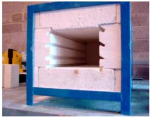
The elements MUST be made from Kanthal wire and are rated at 13 amp, 3.1KW 240V. If you use the same supplier as me you will need two elements wired in series.
