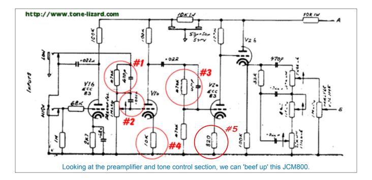
Let us start right at the input jacks. What you should note is the 'High' input is a single gain stage feeding the closed circuit jack labeled 'Low'. The 'Low' input is attenuated by a parallel combination of a 470K resistor and a 470pF capacitor.
