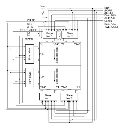
Remark The /DOUT pin is an output pin for the column driver.
