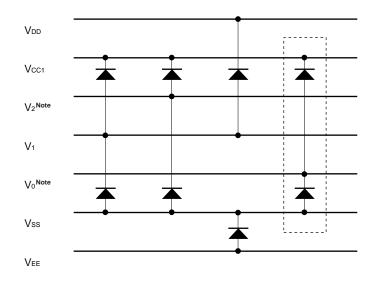
Note  $V_0$  and  $V_2$  are column driver liquid-crystal power supplies.
