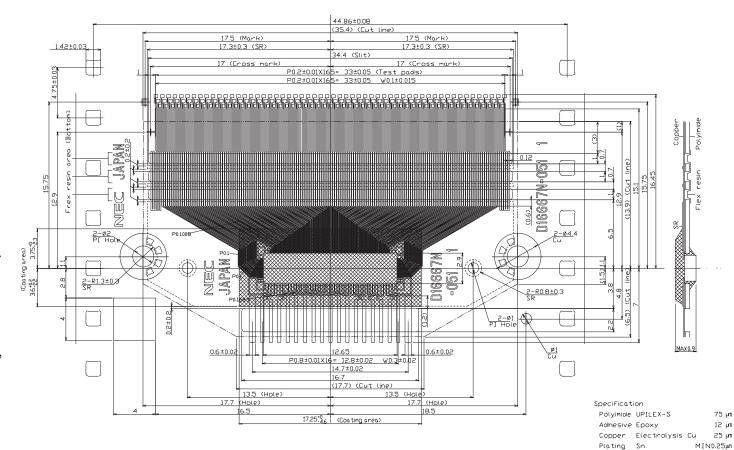
This products is Frex resin type This Figure is shown by Copper side over Polyimide SSprocket holes(23.75 mm)for 1 Pattern Corner radius is 0.30 mm Max. All tolerances unless otherwise specified 0.05 mm.
