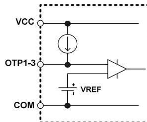
Figure 16 Over Temperature Protection Input Structure
