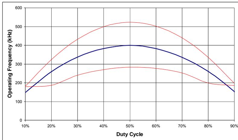
**Figure 5 Typical Lock Range to External Clock**
