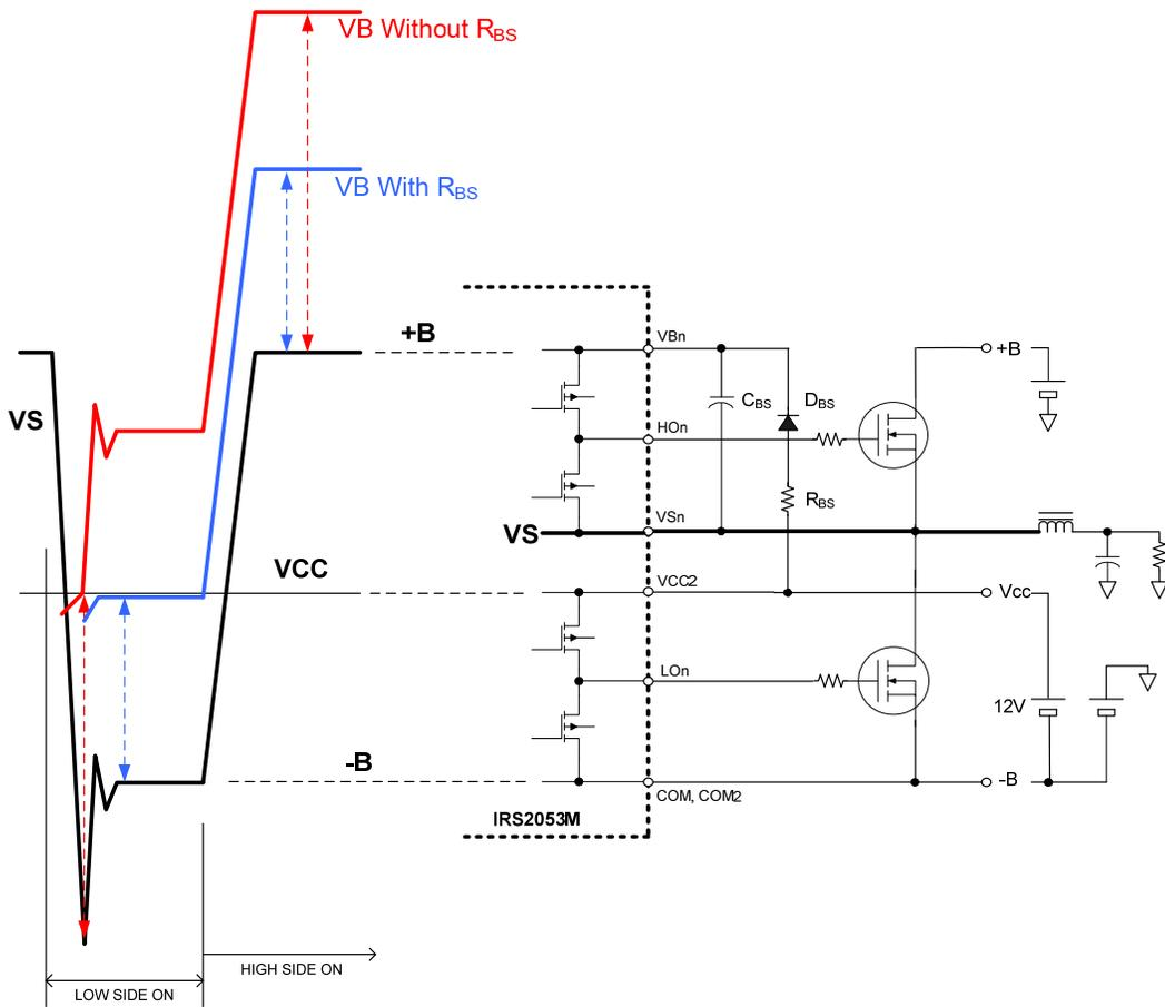
**Figure 29  $V_{BS}$  Charging With and Without  $R_{BS}$**
