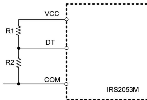
Figure 21 External Voltage Divider for DT Pin
