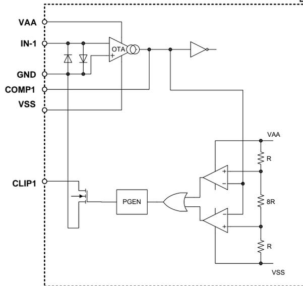
**Figure 18 Clipping Detection**
