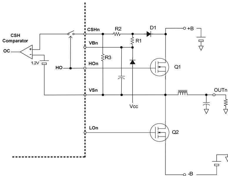
**Figure 15 Programming High Side Over Current Threshold**
