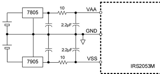
**Figure 22 Supplying  $V_{AA}$  and  $V_{SS}$  with External Regulators**
