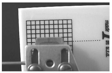
When the cartridge is properly positioned, tighten the cartridge mounting screws and remove the alignment jig. Do not make them overly tight, the 3D arm is self-damping and you can damage the surface by over tightening.
