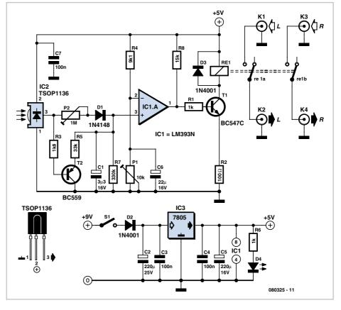
other input on pin 2. This reference voltage, which can be adjusted with P1, determines the switching threshold of the comparator. If IC2 receives an IR signal, T2 conducts, and as a result the voltage on C1 drops rapidly below the threshold level set by P1. This causes T1 to change from its previous 'on' state to the 'off' state. As a result, the relay drops out and the audio link to the stereo system is interrupted for the duration of
