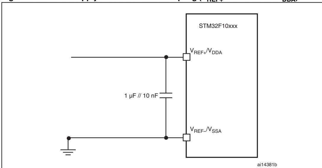
1.  $V_{REF+}$  and  $V_{REF-}$  inputs are available only on 100-pin packages.
