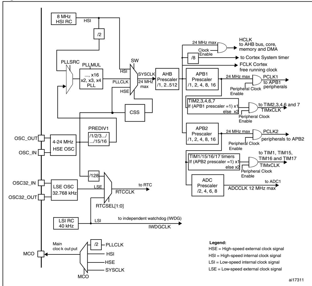
4. To have an ADC conversion time of 1.2 μs, APB2 must be at 24 MHz.
