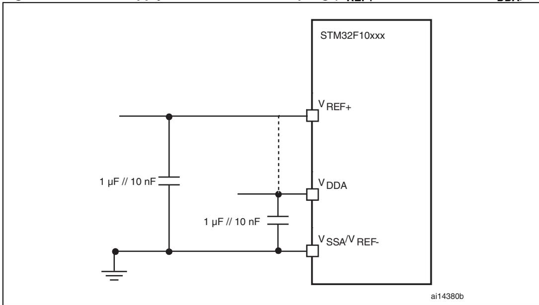
1.  $V_{REF+}$  is available on 100-pin packages and on TFBGA64 packages.  $V_{REF-}$  is available on 100-pin packages only.
