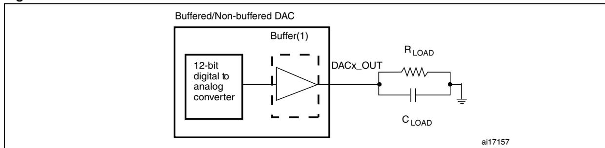
1. The DAC integrates an output buffer that can be used to reduce the output impedance and to drive external loads directly without the use of an external operational amplifier. The buffer can be bypassed by configuring the BOFFx bit in the DAC\_CR register.
