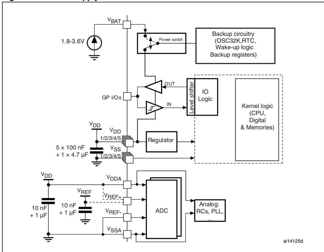
**Caution:** In [Figure 10](#), the 4.7 μF capacitor must be connected to V<sub>DD3</sub>.
