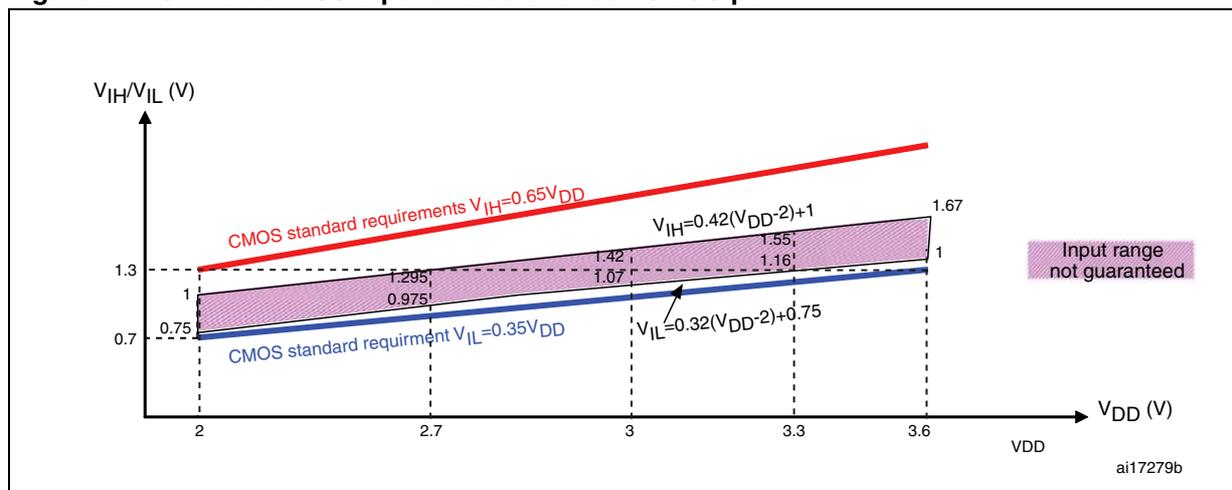
Figure 25. 5 V tolerant I/O input characteristics - TTL port
