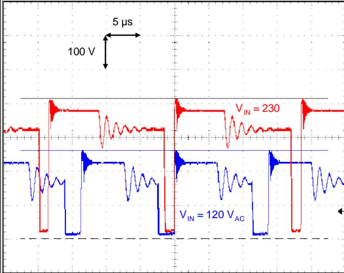
Drain waveform at 120 Vac and 230 Vac
