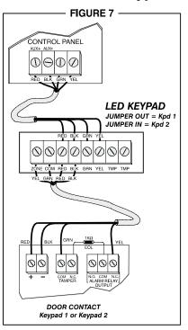
To disable the keypad zone (when keypad zone supervision is deactivated), you must connect a  $1K\Omega$  resistor across the two connections labeled "zone" and "com" on the keypad. (On the 616 keypad, connect the blue wire "zone" to the black wire "com" and remove the EOL jumper 2.)
