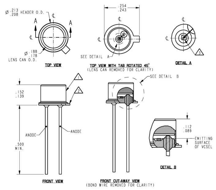
MOUNTING DIMENSIONS (for reference only): All dimensions are in inches. [mm]
