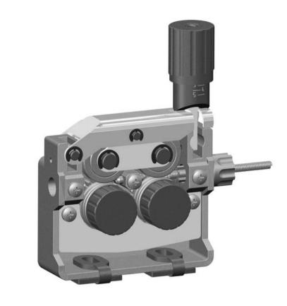
Feeds wire from 0,6 to 2,4 mm (.023"-3/32")
