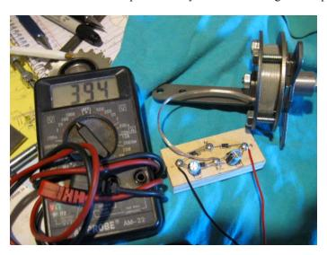
I spun it pretty quick and you can see the voltage reading at 39.4 volts. The capacitors will hold the voltage for a short amount of time which gave me a bit of time to take the above shot.
