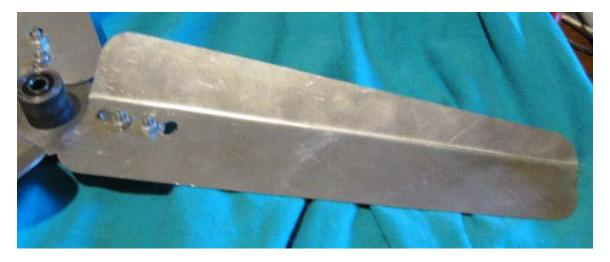
These are 8 inches long, 2 5/8" at the root (attached to the hub) and 1 ½" at the tip. Measured from the trailing edge the bend at the root would be 1 ½" in and the tip would be 1" in. These are inexpensive and quick to make. NOTE: Metal blades spinning fast can be dangerous if you'r not watching what you'r doing. You are, of course, responsible for your own actions when using these or any other spinning attachments with this generator. Safety is your responsibility.
