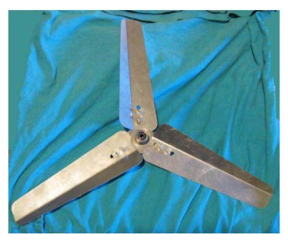
These were made from thin flat aluminum sheet then bent to form the airfoil. Also, by bending them makes them quite strong as well. Below shows a closer look at a single blade...
