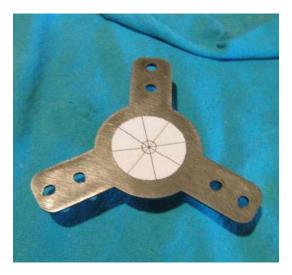
Once centered, use a marker to add extensions to the lines on the hub. Remove the template and connect the lines using a ruler and marker. A fine point marker works well for this.
