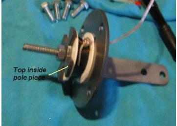
Take the large silicone steel ring and place it over the coil and put the  $4 - \frac{1}{4}$ " x  $\frac{3}{4}$ " bolts through the holes in the base to center it up...
