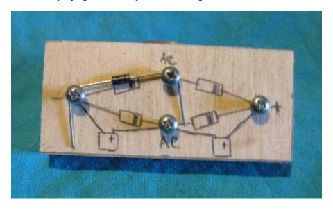
Complete the bend around the screw forming a loop then snip off the excess wire. Continue putting the parts in their appropriate place completing the circuit as in the diagram above.
