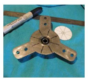
The magnets will be placed on these lines in an alternating pattern. That is to say each magnetic pole will be opposite each other all the way around (i.e. N-S-N-S etc.). The actual north or south pole really doesn't mater as long as their placed in an alternating pattern.
