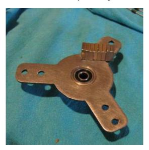
The template on the next page can be used as a guide to mark the magnet placement on the hub assembly. Simply print it and cut it out ....
