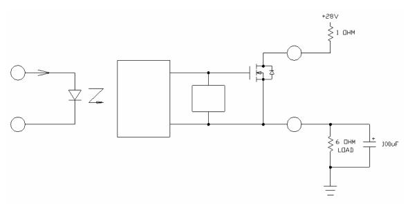
Figure 8.- Surge Current Limiting Using a 1-Ohm Resistor
