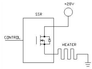
Figure 5.- One of Eight Channels in an RDHA701FP10A8QK Driving a Heater Element on the high side.
