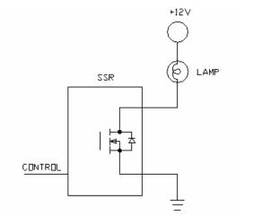
Figure 6.- An RDHA703NM10A1K Driving a Lamp on the Low Side
