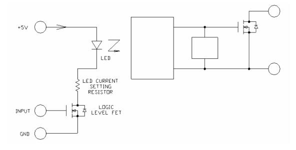
Figure 3.- One type of SSR Input Buffer
