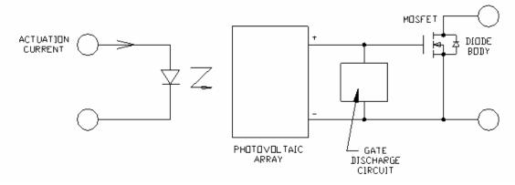
Figure 1.- SPST NO (Form A) DC SSR Circuit Schematic
