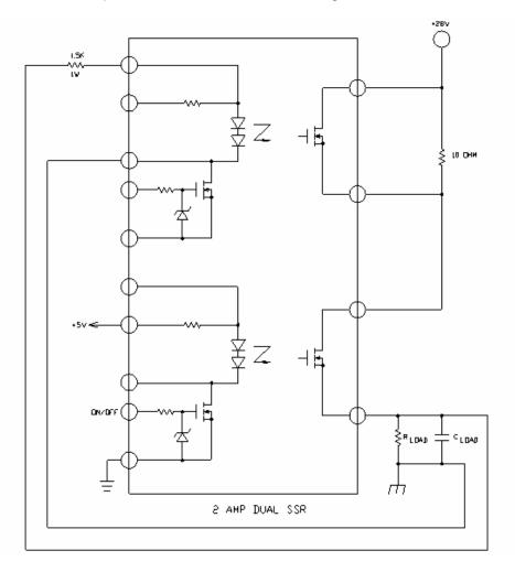
Figure 10.- Automatic bypassing of a current limiting resistor
