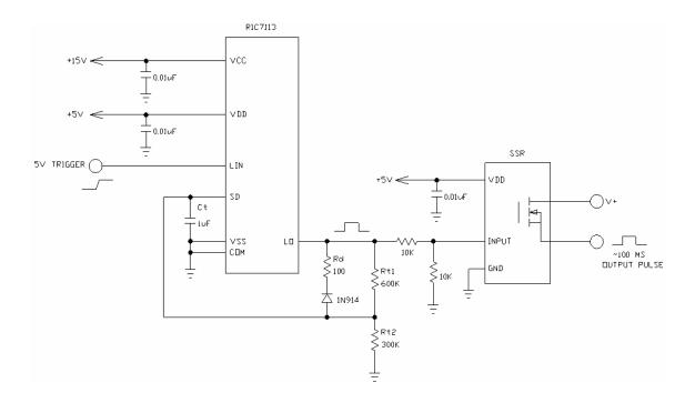
Figure 12.- Rad-Hard Single Shot High Current Pulse Generator
