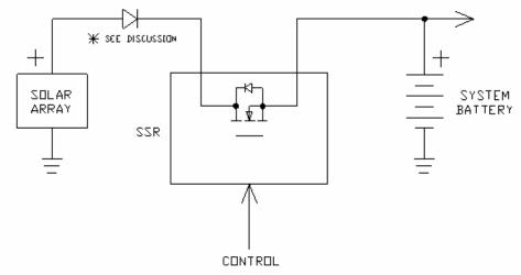
Figure 7.- An RDHA718SE10A2QK Being Used to Control Battery Charging
