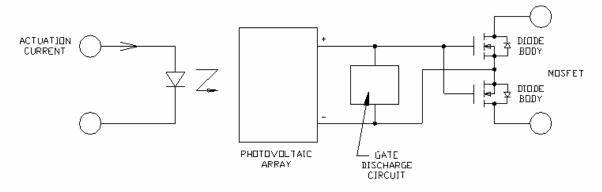
Figure 2.- SPST NO (Form A) AC SSR Circuit Schematic
