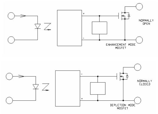
Figure 4.- RDHA718SD10C1BK Single Pole, Double Throw (Form C) DC SSR
