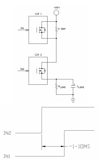
Figure 9.- Sequenced Switching Out of a Current Limiting Resistor
