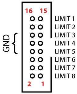
*LIMIT* 1-8 – for connecting limit switches. It is recommended that you put 100nF capacitor directly to key teminals.
