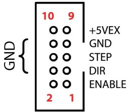
+5VEX - 5V power of motor driver. This pin can be used to power motor driver from controller or to power controller from motor driver. 5VEX jumper on controller must be closed to enable this connection.
