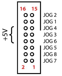
*JOG 1-8* – for connecting jog keys. It is recommended that you put 100nF capacitor directly to key teminals. Typical connection is:
