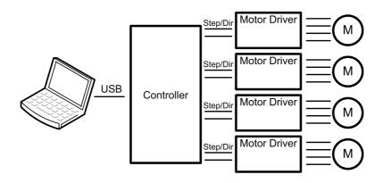
Controller must be connected to motor drivers which drive motors. Computer is connected to USB connector.
