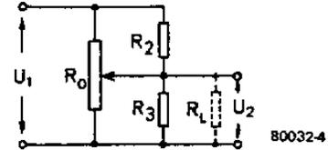
Figure 4. One or two fixed resistors can be added, Between the wiper and one or both of the ends. The results can be surprising!
