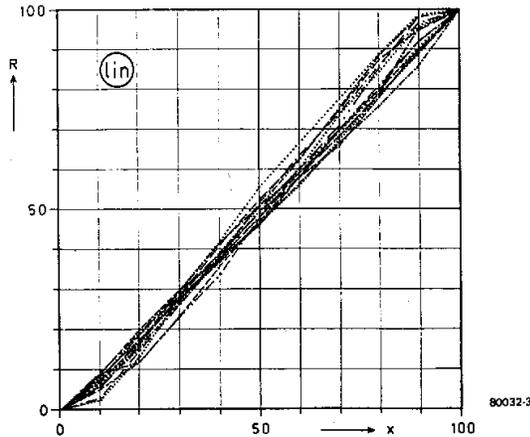
Figure 2. In practise, so-called logarithmic pots may have a wide variety of characteristics. In practice, the desired characteristic is approximated more or less by a series of straight lines.
