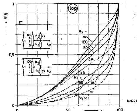
Figure 8. A logarithmic pot and two resistors can produce this intriguing set of plots. As before, the full lines are valid when  $R_2$  is fixed and  $R_3$  is varied And the dotted lines are obtained when  $R_3$  is fixed at  $\frac{1}{4}$  of the total pot value. The basic logarithmic plot is also indicated, as a reference.
