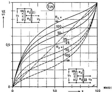
Figure 7. Using two resistors and a linear pot. The full Lines correspond to the situation where  $R_2$  is fixed, And equal to  $\frac{1}{4}$  of the total pot value; the dotted Lines are obtained when  $R_3$  is fixed and  $R_2$  is varied.
