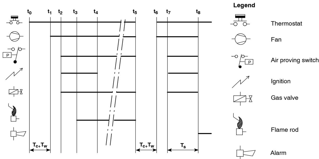
Fig. 11. Functional diagram S4565CM, DM, RM, TM
