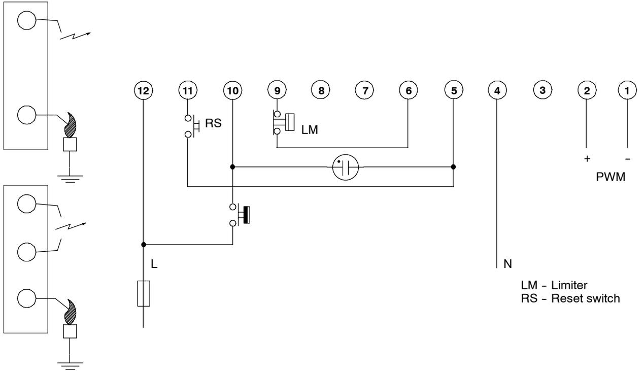
Fig. 4. Connection diagram S4565AM, BM, PM, QM <sup>1)</sup>
