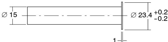
**Fig. 19. Pipe (dia 15 mm) for flat sealing ring connection for G 3/4" external thread**
