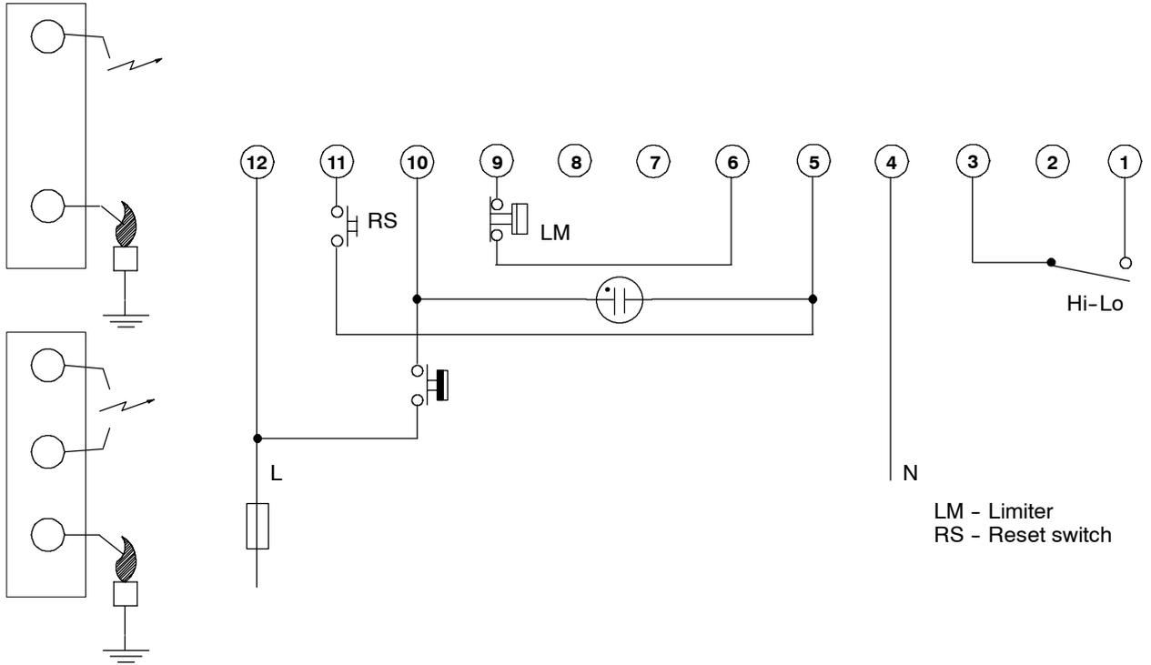
Fig. 8. Connection diagram S4565BM, QM with Hi-Lo <sup>1)</sup>
