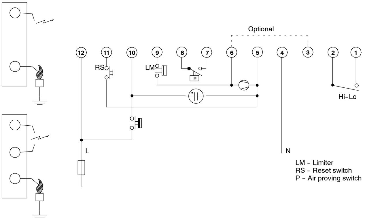
Fig. 7. Connection diagram S4565CM, RM with Hi-Lo <sup>1)</sup>
