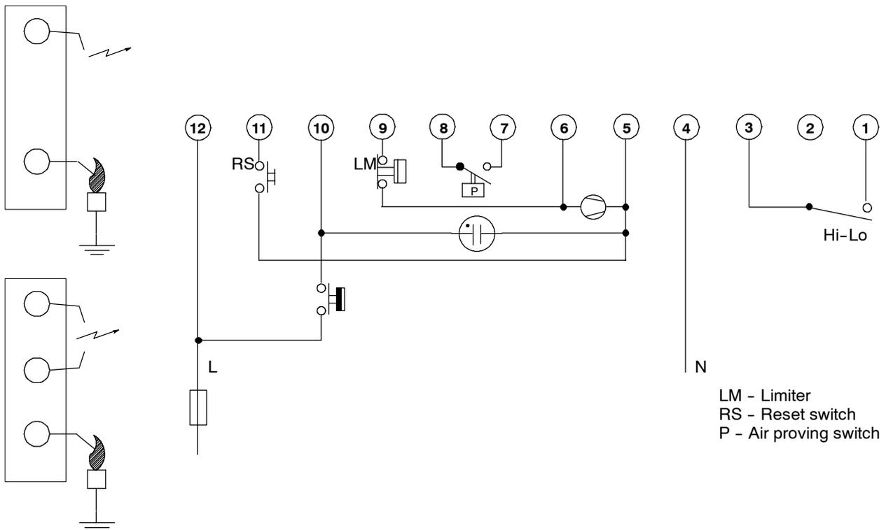
Fig. 9. Connection diagram S4565DM, TM with Hi-Lo <sup>1)</sup>
