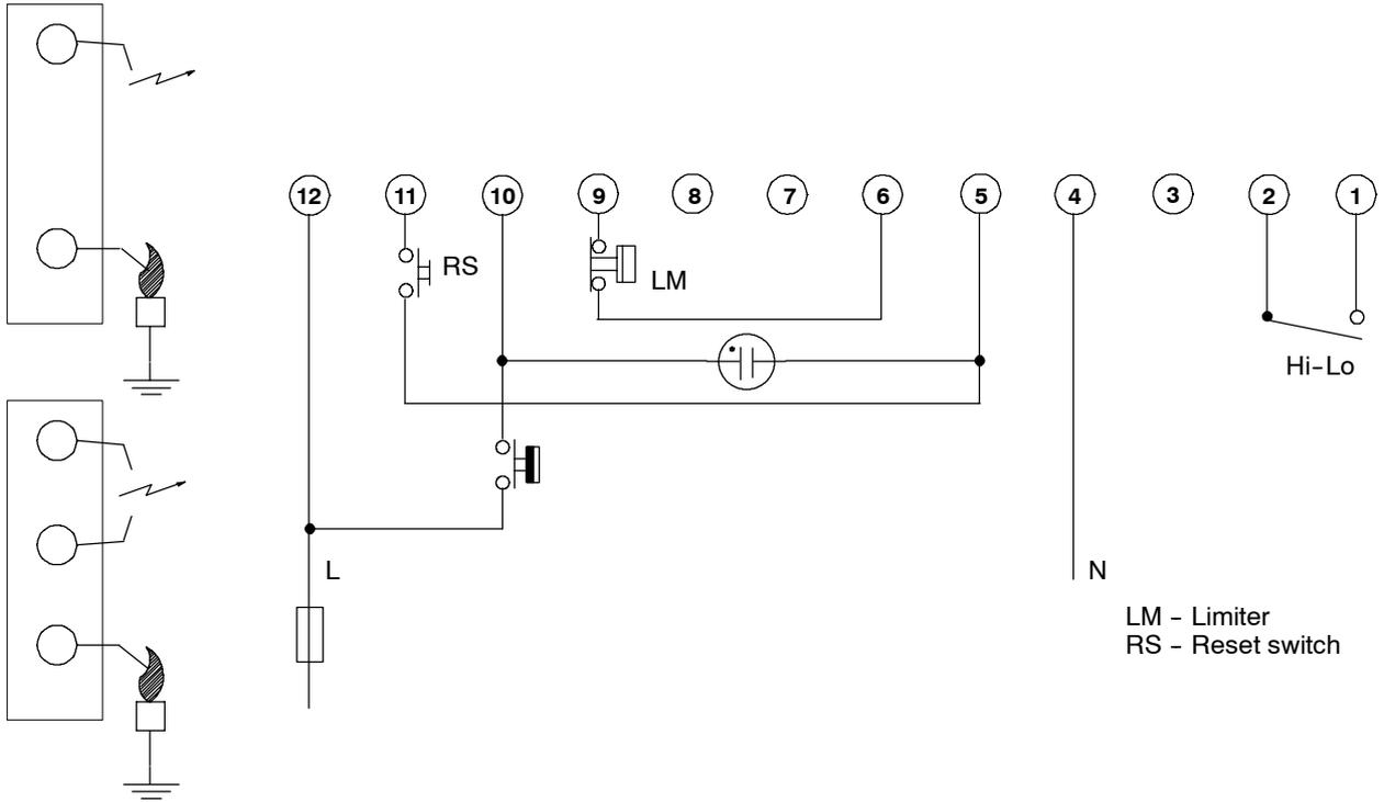
Fig. 6. Connection diagram S4565AM, PM with Hi-Lo <sup>1)</sup>
