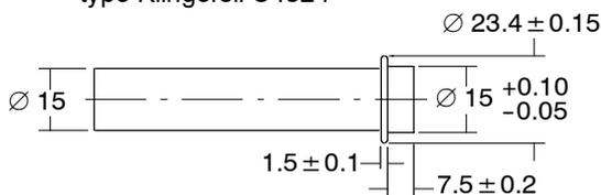
**Fig. 18. Pipe end for "O"-ring connection for G 3/4" external thread**
