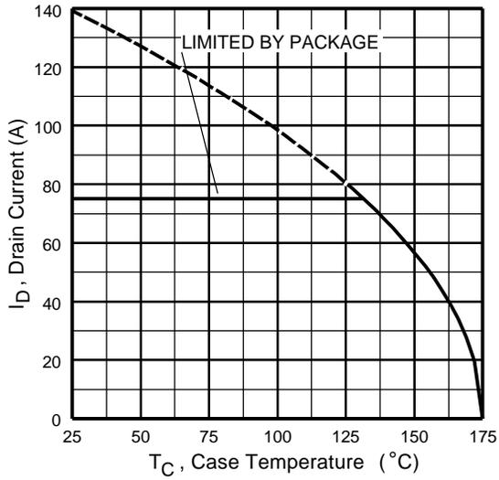
Fig 9. Maximum Drain Current Vs. Case Temperature
