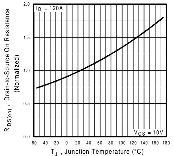
**Fig 4.** Normalized On-Resistance
