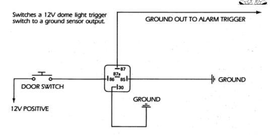
The door switches can be motion sensors, shaker boxes, glass sensors...etc., any trigger you wish to invert.
