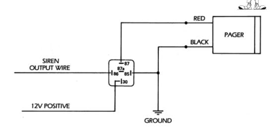
On some import or older model cars, the vehicle's ignition or charging system can cause noise to be picked-up by high end audio systems or cellular phones. To eliminate this noise, use the following diagram.
