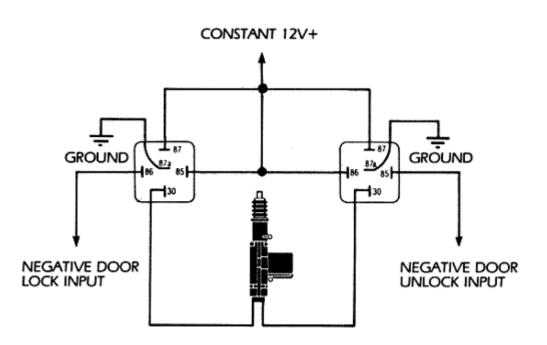
Negative door lock and unlock output reversing polarity
