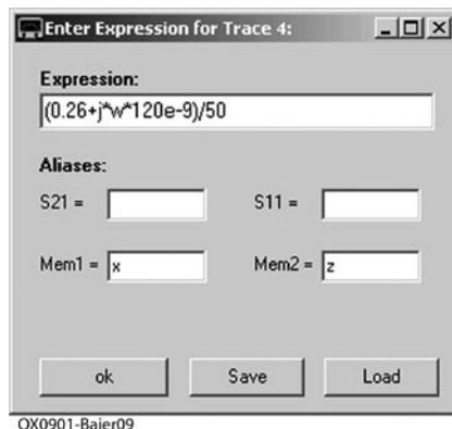
**Figure 9** — VNWA software input mask showing the impedance formula of the lossy 120 nH inductor normalized to 50 Ω used in the simulation trace 4 of Figure 8.
