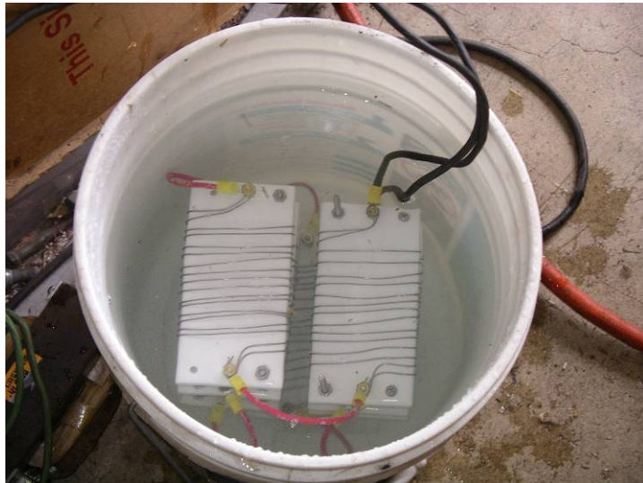
Figure 7: Resistors immersed in water.
