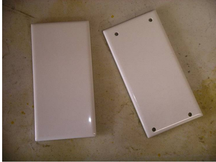
Figure 4: Ceramic tiles used for making resistors
