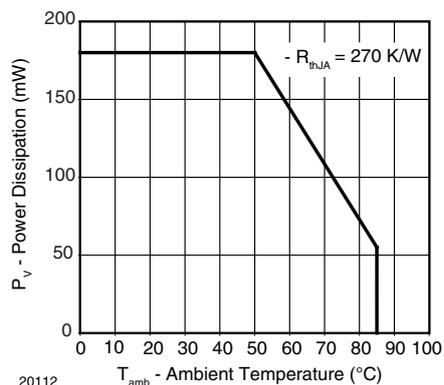
Figure 1. Power Dissipation Limit vs. Ambient Temperature
