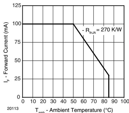
Figure 2. Forward Current Limit vs. Ambient Temperature
