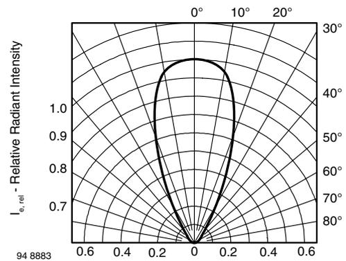
Figure 8. Relative Radiant Intensity vs. Angular Displacement
