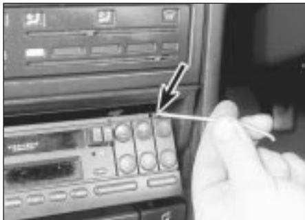
20.13 Make up two removal tools - note slot (arrowed) in end of tool
