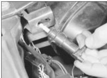
7.4 Removing a cable-operated headlight adjuster
