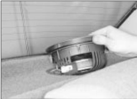
**21.13 Removing the rear loudspeaker - Saloon models**
