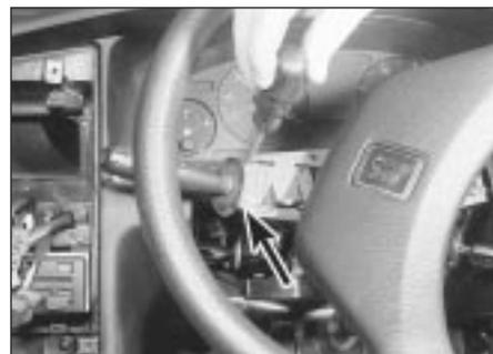
4.6a Remove the securing screws . . .
