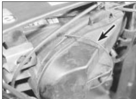
5.2 Headlight rear cover securing clip (arrowed)
