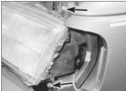
7.8 Outer headlight securing bolts (arrowed)
