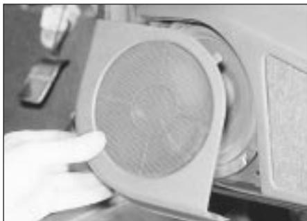
21.2b . . . and remove loudspeaker cover panel from the door - models up to 1992
