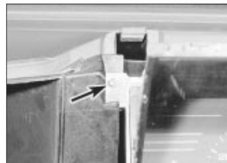
9.8 Instrument panel securing screw (arrowed)
