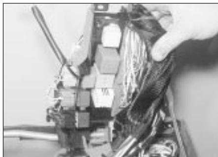
3.14c Main relay box located behind fusebox at rear of facia - models from 1993 (viewed with facia removed and inverted)
