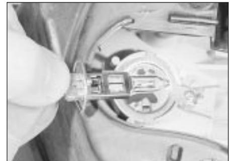
5.23b Removing a headlight-mounted driving light bulb
