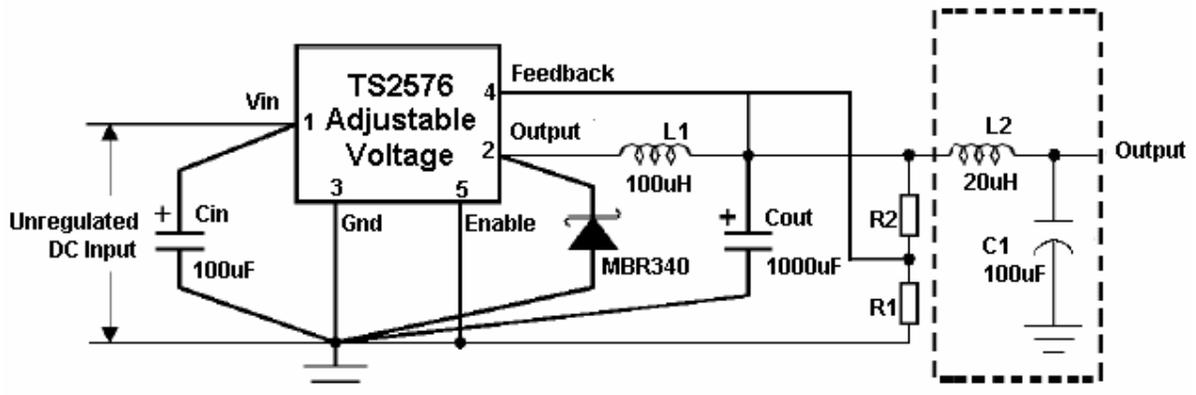
Figure 3: LC filter for Low Output Ripple
