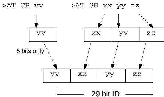
Figure 5. Setting a 29 bit CAN ID
