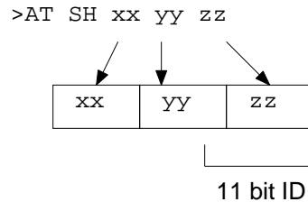
Figure 6. Setting an 11 bit CAN ID
