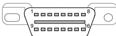
Figure 7. The J1962 Vehicle Connector
