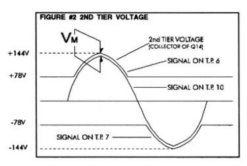
3.5v)) then Q11 will start to turn on the second tier. The second tier voltage will remain about 11 volts (Vm) above the peak of the output signal to the point of clipping where this voltage is reduced to about 4 volts. Zener ZD8 protects the gate source junction of Q11 and also provides a current path through R29 for the "floating battery".
