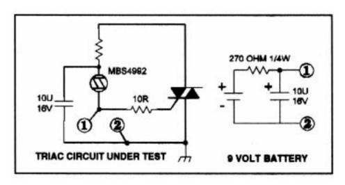
**NOTE:** Everytime you replace blown output transistors on a M1002A board test the DC protection triac with the following circuit.
