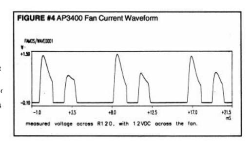
providing the drive current for the fan. To lower the dissipation of Q35, D42, D43, ZD12, ZD13 and R118 turn off Q35 when the full wave rectified voltage present of the collector of Q35 reaches approximently 50V by robbing current from the base of Q34. The maximum fan voltage is 20.5 VDC. ZD14 and R120, R121 and R122 provide a current limiting function. Figure #4 shows the current throught these resistors when there is 12VDC across the fan.
