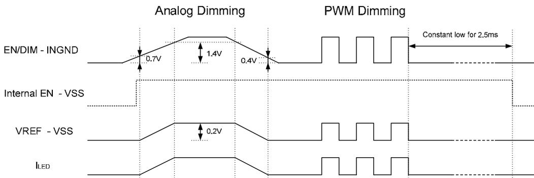
**Figure 2— Internal EN Shut-down Delay Function Waveform Diagram**
