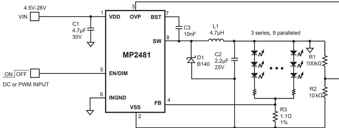
**Figure 4—Step-up/down White LED Driver Application**
