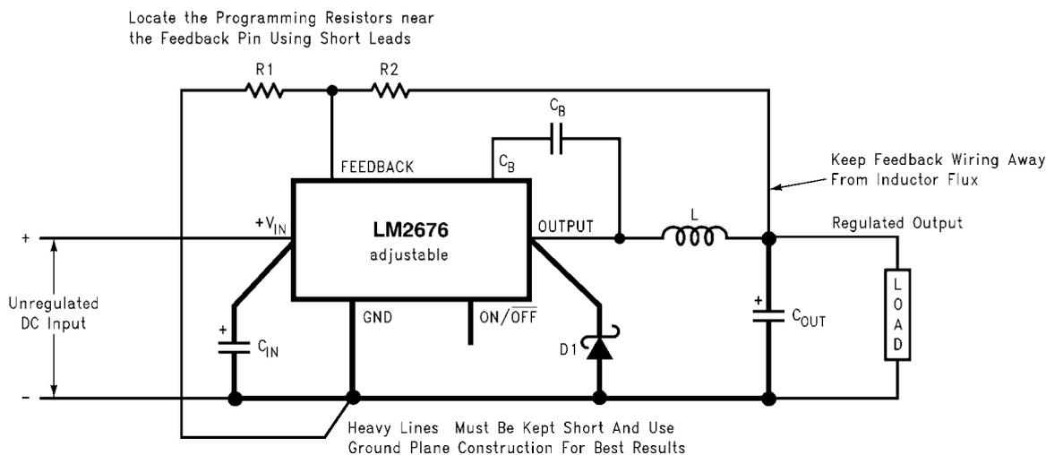
FIGURE 2. Basic circuit for adjustable output voltage applications
