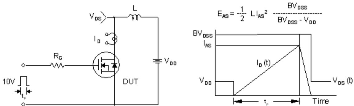
Peak Diode Recovery dv/dt Test Circuit & Waveforms
