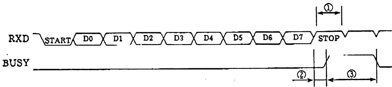
①  $t(\text{DATA}) = 106 / \text{baud rate} [\mu\text{s}]$
