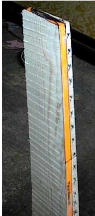
**Now grab a hammer and a wood chisel and start making chips... This goes fairly fast but you have to be careful and watch the grain of the wood. You don't want to split into the marked area. On the larger chunks where the cuts went deeper you should take them down a little at a time. I usually start from the tip and work my way down to the root as shown below...**
