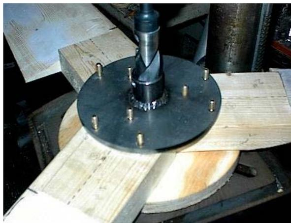
If you don't have a 1 inch drill you can mark the point on the root at  $\frac{1}{2}$  inch up toward the tip straight across and this will accomplish the same thing. No more than  $\frac{1}{2}$  inch though, it's best to allow the wood to sit on the shaft. You can hone the hole with a larger drill with some sandpaper
