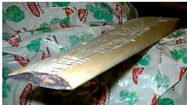
**For the trailing edge of the airfoil I used a full size plane to remove the material fairly quickly also shown in the above picture. That is the rough airfoil shape. You can use the pocket plane to shave down the lines and remaining chunks left before starting the sanding process.**
