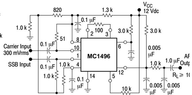
Figure 28. Product Detector (12 Vdc Single Supply)
