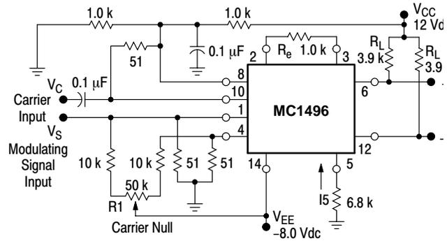
Figure 26. Balanced Modulator-Demodulator
