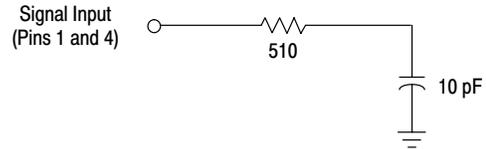
An alternate method for low-frequency applications is to insert a 1.0 kΩ resistor in series with the input (Pins 1, 4). In this case input current drift may cause serious degradation of carrier suppression.
