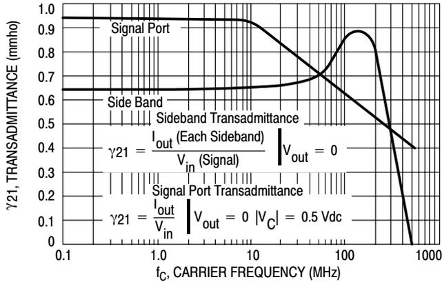
**Figure 15. Sideband and Signal Port Transadmittances versus Frequency**
