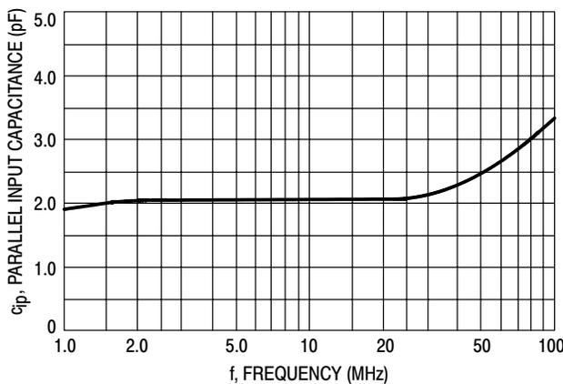
Figure 13. Signal-Port Parallel-Equivalent Input Capacitance versus Frequency
