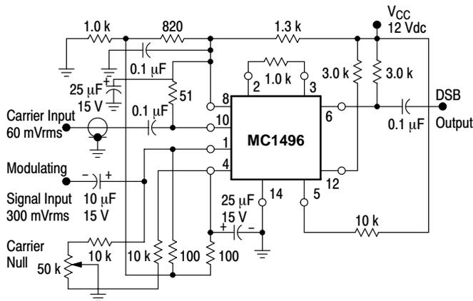
Figure 25. Balanced Modulator (12 Vdc Single Supply)
