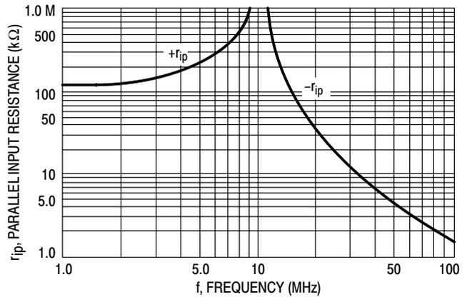
Figure 12. Signal-Port Parallel-Equivalent Input Resistance versus Frequency
