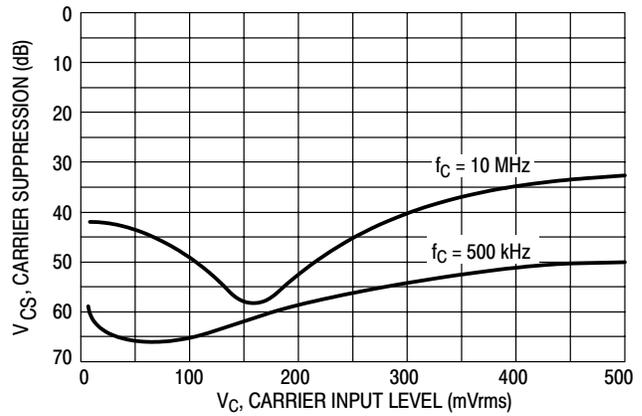
**Figure 22. Carrier Suppression versus Carrier Input Level**
