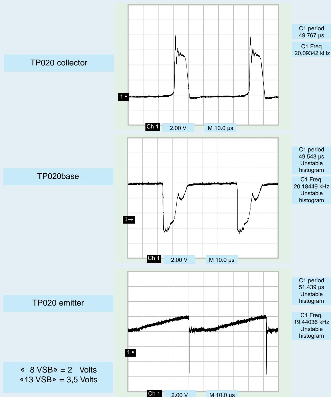
NB. If nothing happens, disconnect the collector of TP020 and check the presence of about 2V6 at the cathode of the Zener diode DP019.
