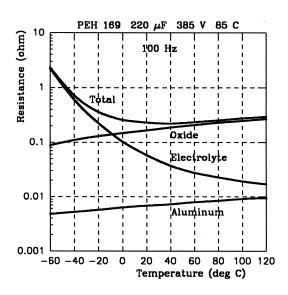
End of life of the capacitor is defined when one or more of the capacitor parameters have changed by a given amount. Those parameters are capacitance (C), ESR, dissipation factor (DF), and leakage current (I<sub>L</sub>). Different manufacturers define those limits differently depending on their capacitor capabilities. Evox Rifa defines end of life of their electrolytic capacitors when,
