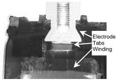
laser welding that Evox Rifa developed, more tabs can be added and hence lower ESR can be achieved. This means more ripple current capability and less internal heating which means longer life.
