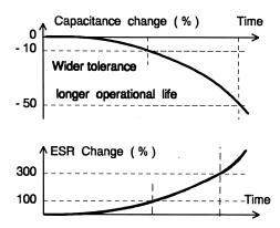
$\Delta C = 15\%$  for  $V_r \le 160$  VDC ( $V_r = Rated Voltage$ ). 10% for  $V_r > 160$  VDC.
