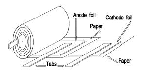
In the non-solid electrolytic capacitor, the dielectric is the oxide layer of the anodic foil. The electrolyte acts as the electric contact between the cathode foil and the oxide layer of the anode foil. Paper layers absorbing the electrolyte acts as a spacer between the cathode and anode foils. The foils are connected to the capacitor terminals by aluminum tabs.
