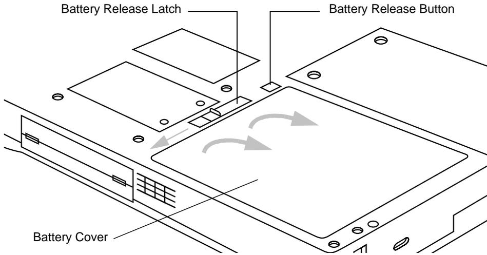
*Figure 2-1 Removing the Battery Pack*
