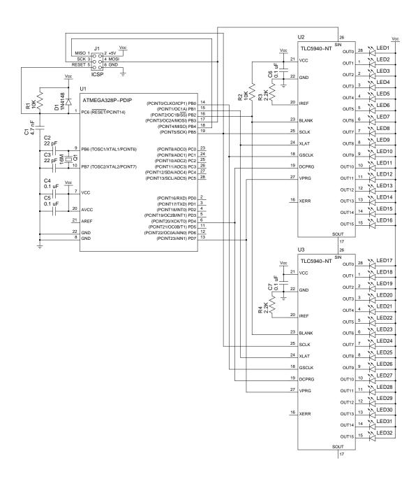
Figure B.1: Connecting two TLC5940 chips in series
