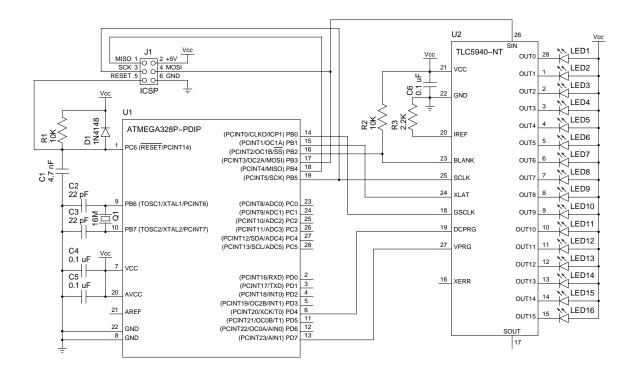
Figure 2.1: Connecting a TLC5940 to an ATmega328P
