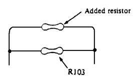
Note: When soldering the resistor (22 kohms) to the resistor R103, try to do it as quickly as possible. After that, touch them by hand to see if they have been secured perfectly.
