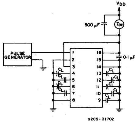
Fig. 14 - Dynamic power dissipation test circuit for CD4033B.
