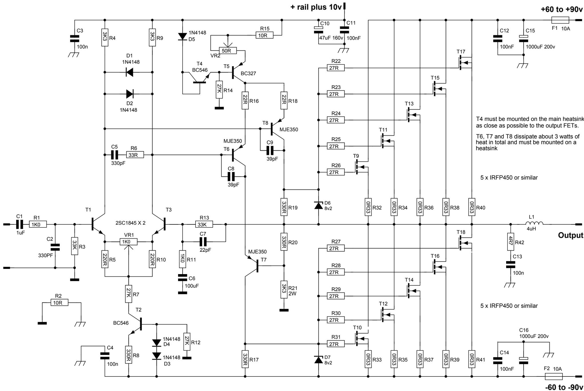
T4 must be mounted on the main heatsink as close as possible to the output FETs.
