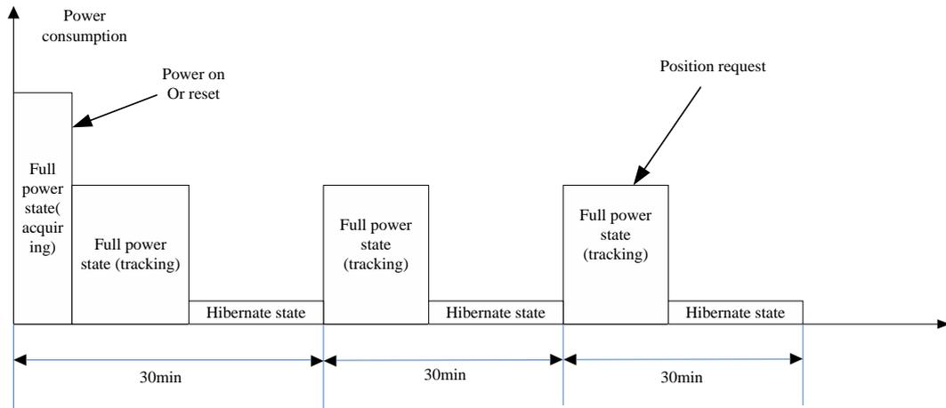
**Figure 3: PTF timing sequence**
