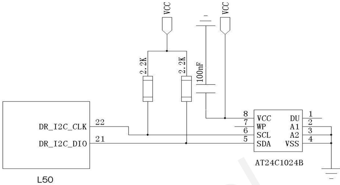
Figure 13: Reference design for CGEE function
