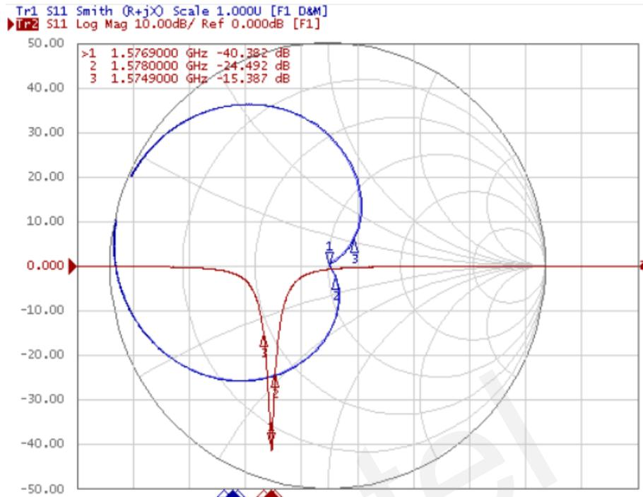
Figure 14: Patch antenna test result with ground plane 29.5mm×28.5mm
