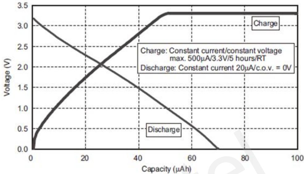
Figure 6: Seiko XH414 charging and discharging characteristics
