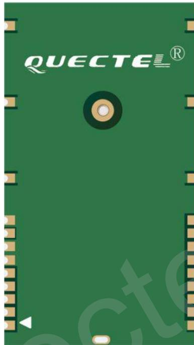
Figure 20: Bottom view of module
