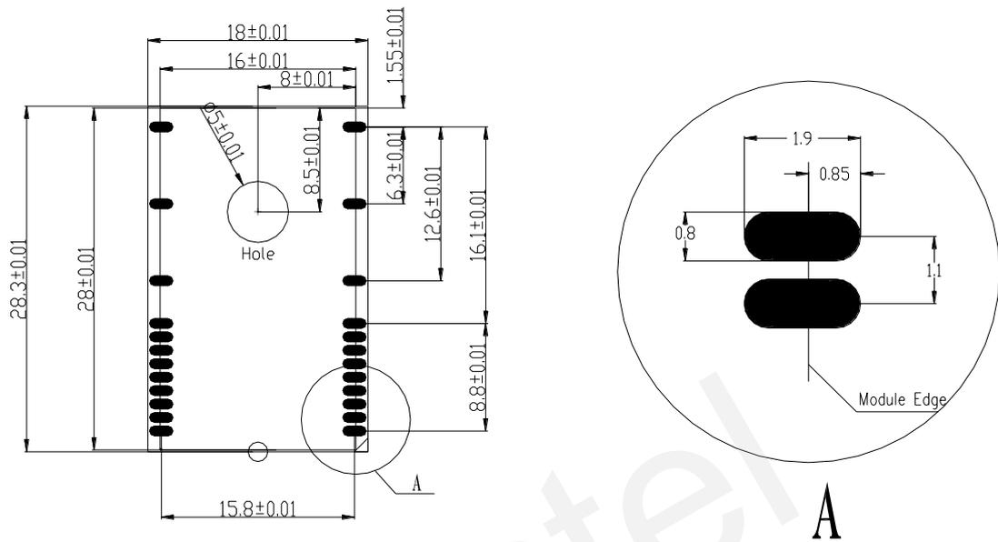
Figure 18: Recommended footprint (Unit:mm)
