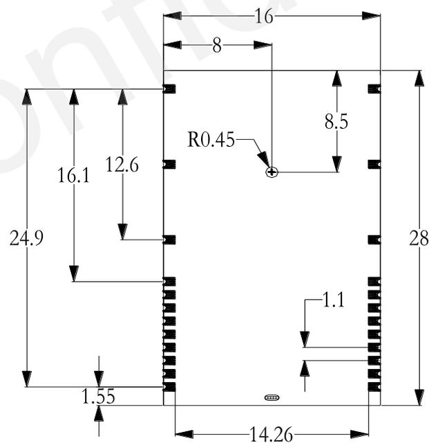
Figure 17: L50 Bottom view (Unit:mm)
