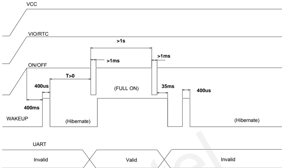
Figure 7: Turn on timing sequence of module
