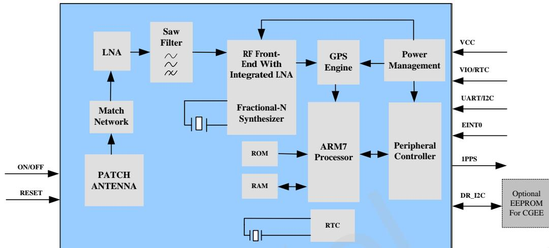
Figure 1: Functional diagram for L50
