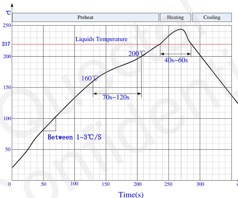
Figure 21: Ramp-soak-spike-reflow of furnace temperature
