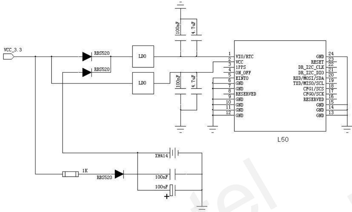
Figure 4: Power design reference for L50 module
