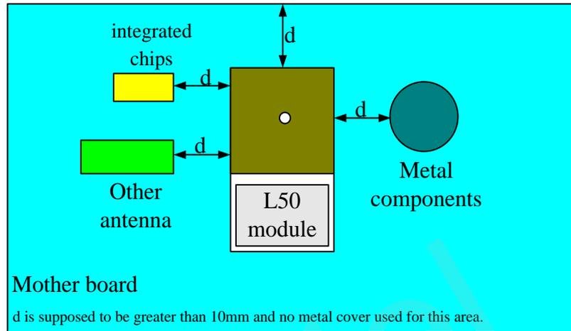
Figure 15: L50 module placement guide
