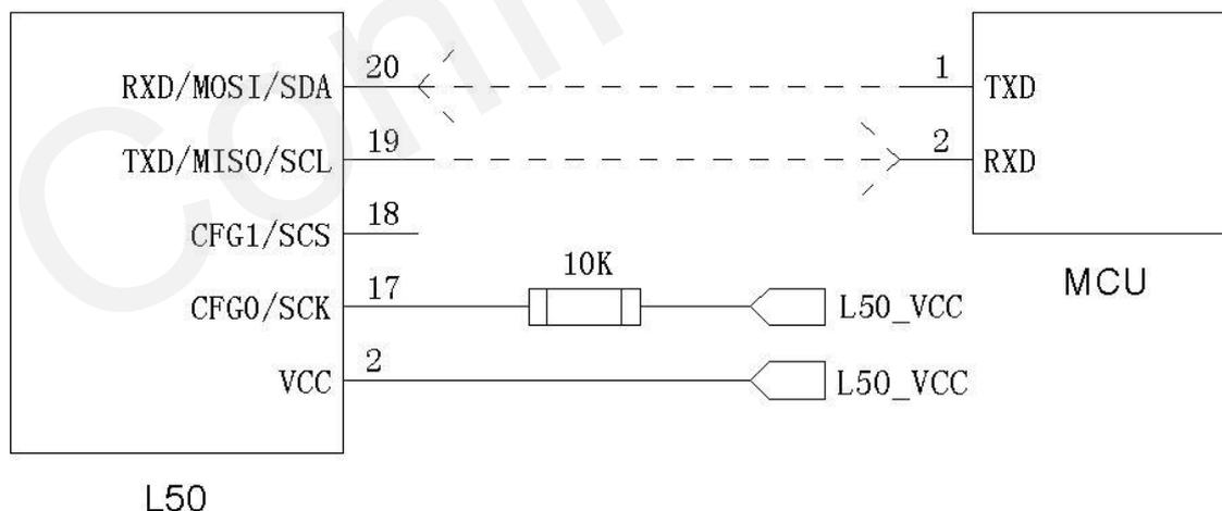
**Figure 9: UART design reference for L50 module**
