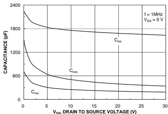
Figure 8. Capacitance Characteristics.
