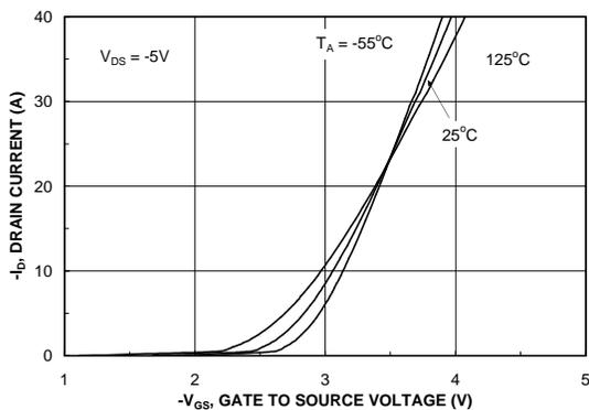
Figure 5. Transfer Characteristics.
