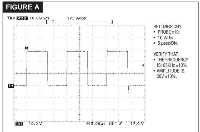
**N.B.** If this signal is absent it may be necessary to replace component Q4 (fig. 3).
