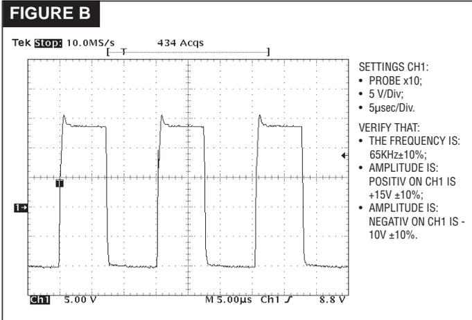
F) Repeat this test on Q5 as well using the differential probe.
