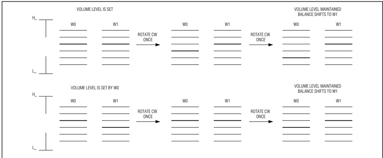
Figure 3. Balance-Control Operation
