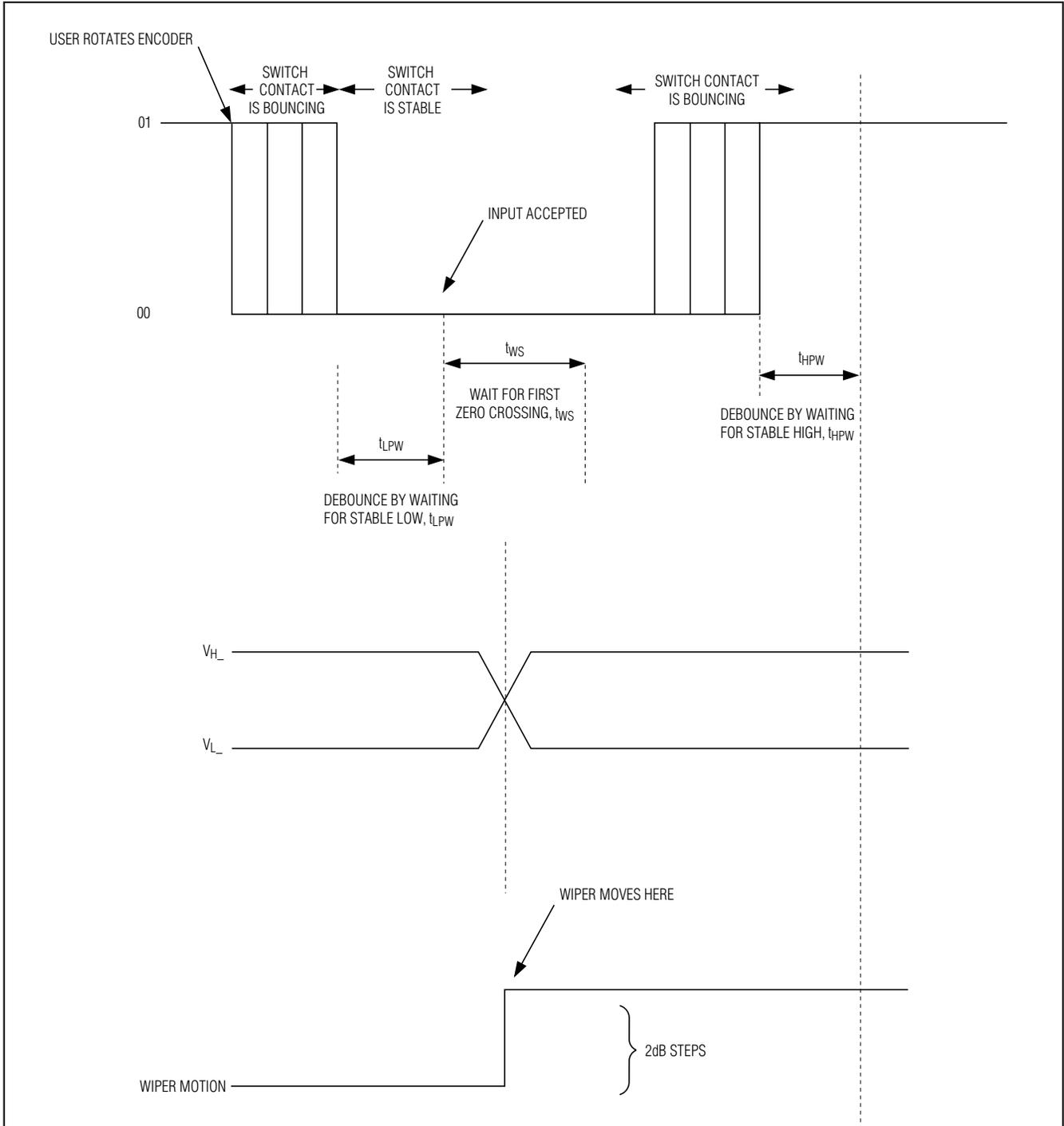
Figure 4a. Wiper Transition Timing Diagram—Suppression Circuitry Active
