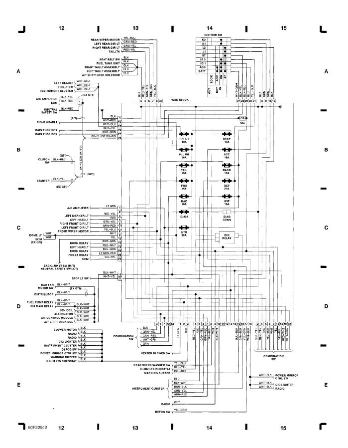
WIRING DIAGRAMS Fig. 5: A/C & Heater, Comb Switch (Grid 16-19) (p. 5) 1990 Suzuki Swift
