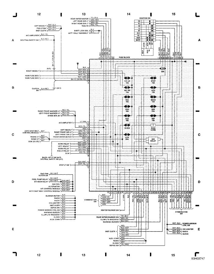
Fig. 5: A/T Ctrl Mod, A/C Amp, Combo Sw, Heater/Blower (Grid 16-19) (p. 5) 1992 Suzuki Swift
