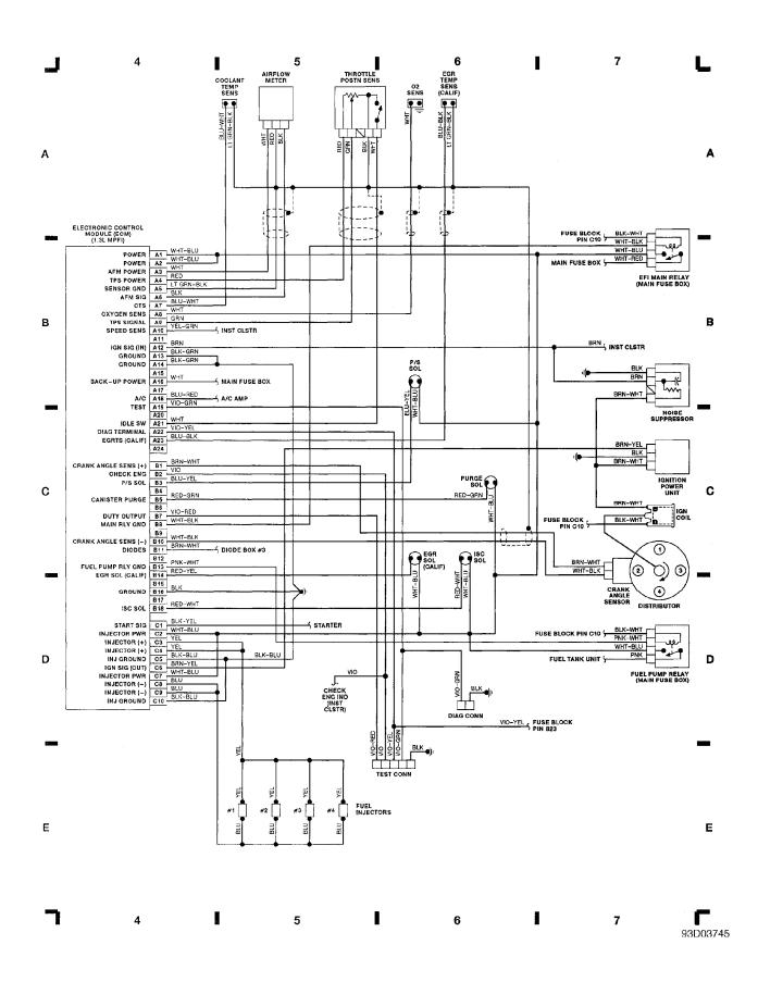
Fig. 3: ECM (1.3L), Engine Sensors, Fuel Pump Relay (Grid 8-11) (p. 3) 1992 Suzuki Swift
