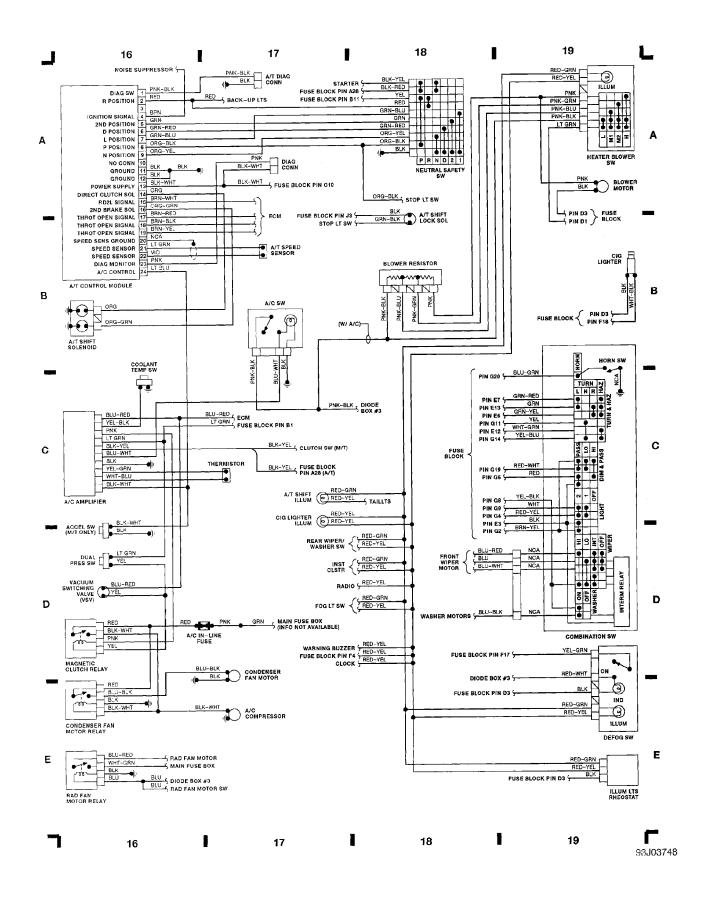
Fig. 6: Instrument Clstr, Seat Belt Ctrl Mod, Clock (Grid 20-23) (p. 6) 1992 Suzuki Swift
