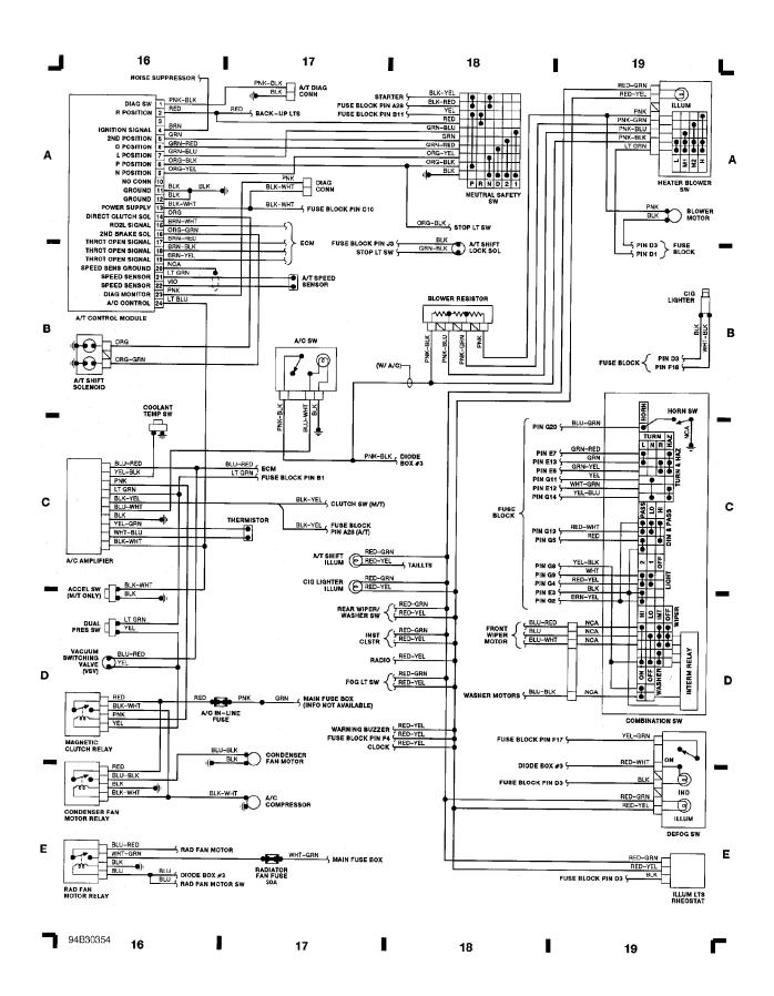
Fig. 6: Instrument Clstr, Seat Belt Ctrl Mod, Clock (Grid 20-23) (p. 6) 1993 Suzuki Swift
