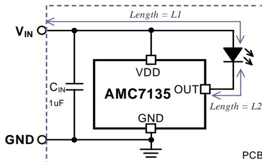
If LED and AMC7135 is located in separate PCBs, or the length of the routing path  $L1 > 10\text{cm}$  or  $L2 > 3\text{cm}$ , the output capacitor  $C_O$  should be added. Typically, capacitance of  $0.1\mu\text{F} \sim 1\mu\text{F}$  is recommended and  $1\mu\text{F}$  is needed when  $L2$  is much longer than  $3\text{cm}$ .
