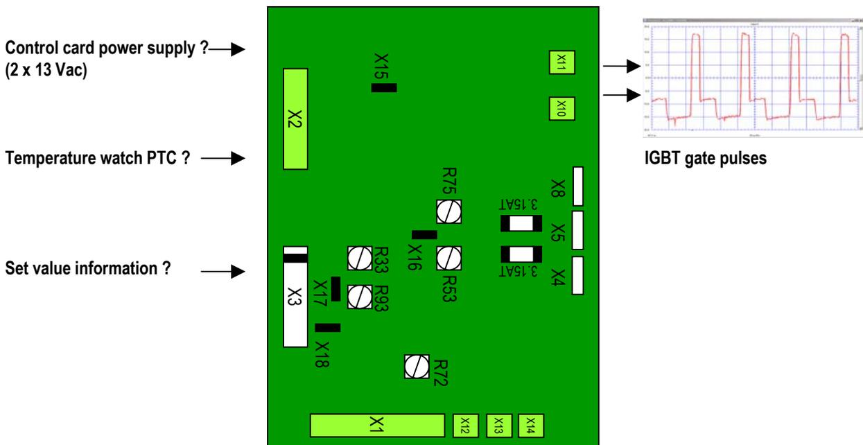
Control card A001 develops the IGBT gate pulses. If the power supply part is OK, the fuses are intact, the temperature watch PTCs are OK and correct set value info is received from the potentiometer, then the gate pulses should be seen on connectors X10 and X11. When the machine is idling, one must note that it is actually running intermittently.
