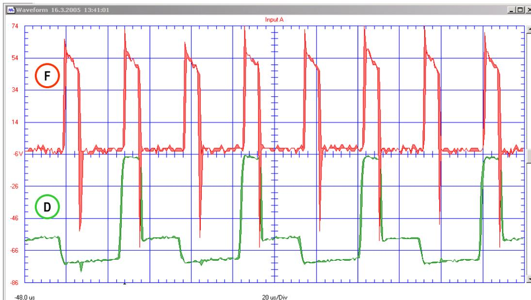
Voltage after the secondary diodes (measuring point F) and lower IGBT gate pulse (measuring point D).
