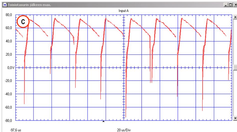
Voltage over the secondary diodes with maximum power (2800/3500). Frequency approx. 38 kHz (measuring point C).
