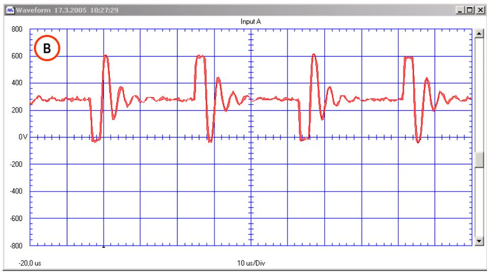
Voltage over the lower IGBT with minimum power (2800/3500). Inverter operating frequency approx. 19 kHz (measuring point B).
