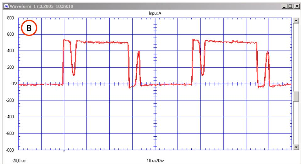
Voltage over the lower IGBT with maximum power (2800/3500). Inverter operating frequency approx. 19 kHz (measuring point B).
