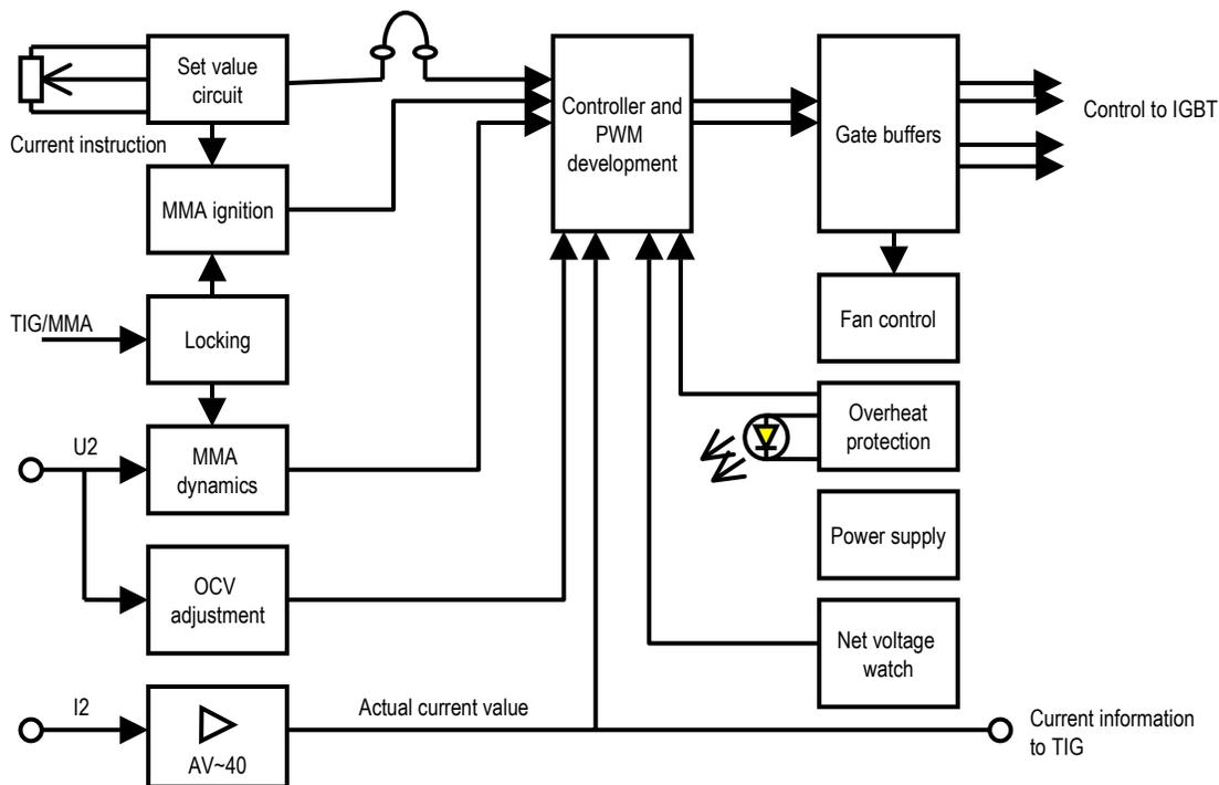
The functions of power source's control card A001 are built around the PWM-controller SG 3526.
