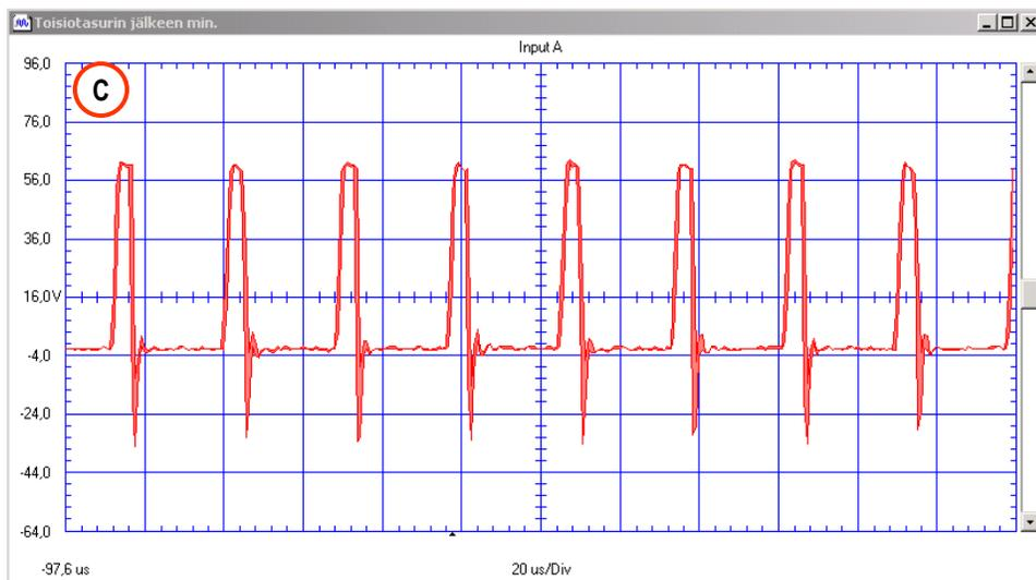
Voltage over the secondary diodes with minimum power(2800/3500). Frequency is approx. 38 kHz (measuring point C).
