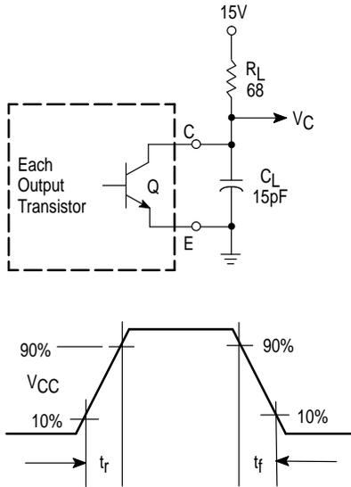
Figure 13. Emitter-Follower Configuration Test Circuit and Waveform
