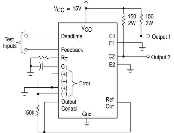
Figure 12. Common-Emitter Configuration Test Circuit and Waveform
